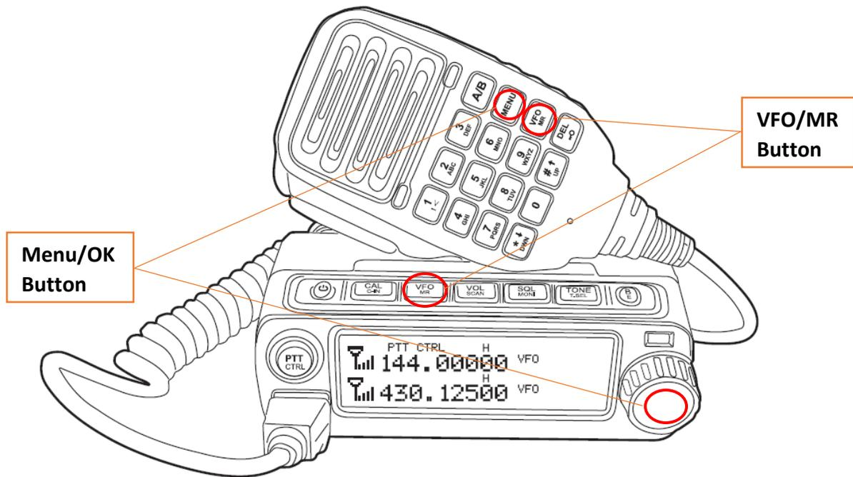
For manually programming the NCR2 radio, you can store up to 255 channels and customize each by name, each channel can be programmed by the following instruction:
